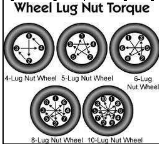
Figure 6-1 Lug nut sequence of tightening
